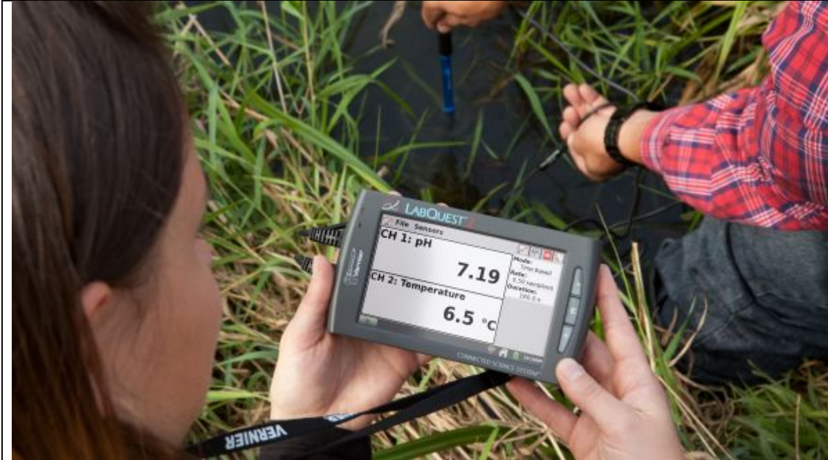
Fig. 7. Stock image showing use of Vernier probe “Labquest” for recording water quality parameters.
